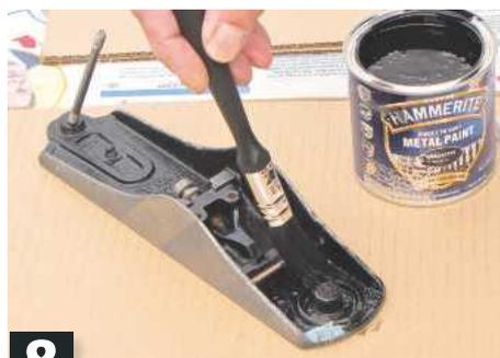
**8** Brush on two coats of Hammerite to painted areas of body (no primer or undercoat needed)
